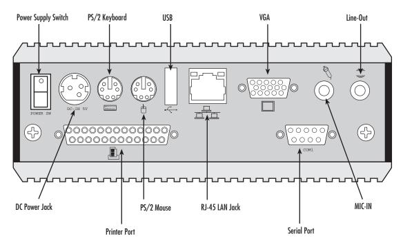
Figure 9. Thin System rear connectors
